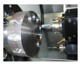
: Max.4000 min-1 Spindle speed Spindle motor : 4.5 kw [ 6.0 hp ] Collet size : AR32 Max. clamping tool dia. : 20 mm [ 0.8 inch ]
